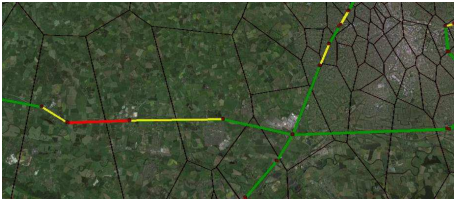
Figure 1: Example of overlap between the cells of the cell-phone network and the links.
